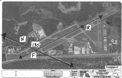
Part A. Flying to the runway from point F, the runway is Runway 13. This means the heading is 130° off magnetic north. Draw a line through point R to that goes to magnetic north, what is true about that line and line NF?
